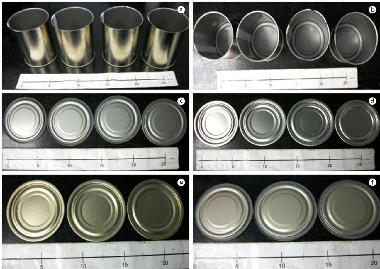
**Figure 1.** Container bodies with yellow stain (a) Exterior (b) Interior. Can lids without blemish (c) Bottom side (d) Upper side. Tops with blemish (e) Bottom side (f) Upper side. The reference is in cm.
