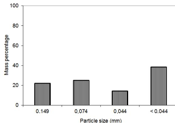
Figure 1. Particle size distribution of the anthracite used in the pelletization.
