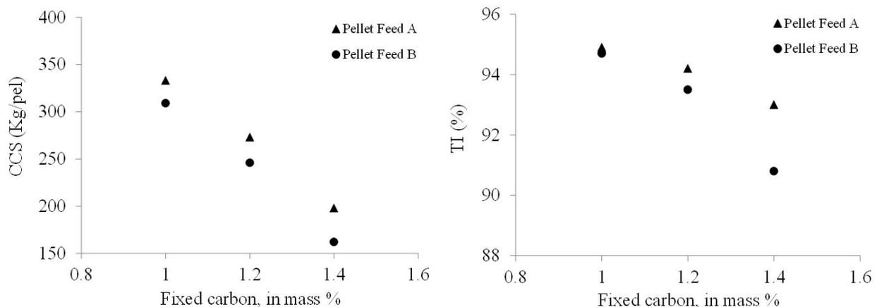
**Figure 2.** Influence of the fixed carbon content on cold compressive strength (a) and on tumbler index (b) of the fired pellets.
