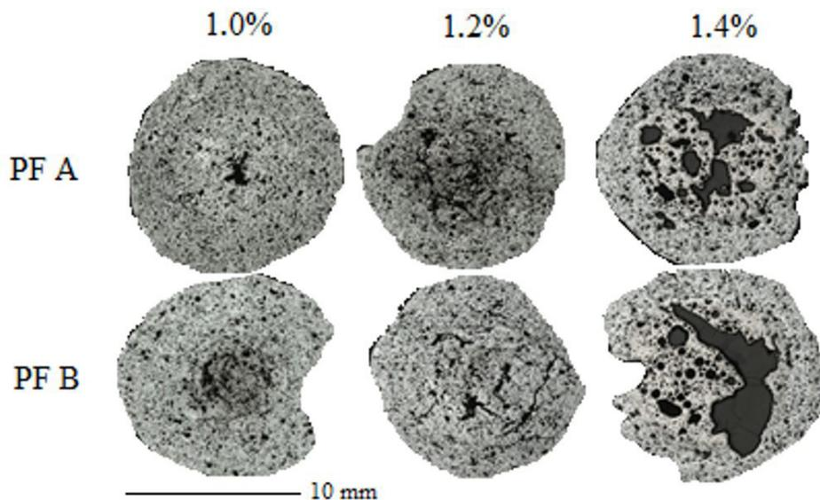
**Figure 3.** Micrograph of the pellets obtained with different fixed carbon content.
