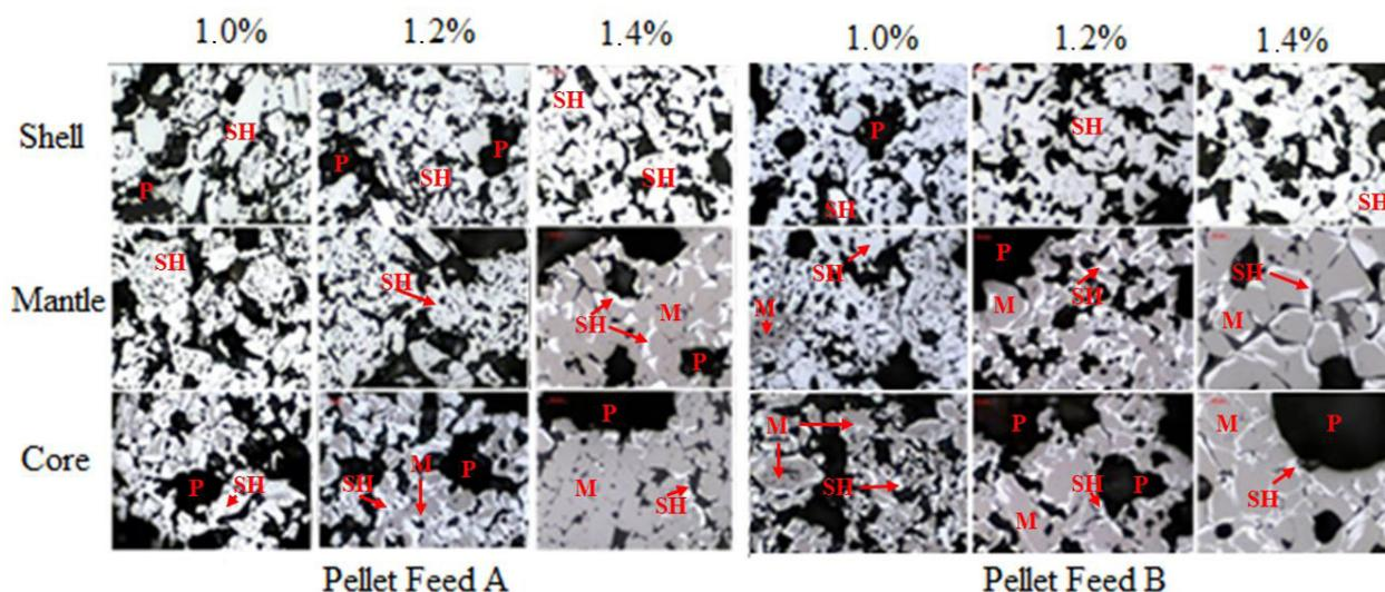
**Figure 4.** Micrographs (magnification 500x) of pellets produced with different mass percentage of anthracite and pellet feed type. SH = secondary hematite; M = magnetite; P = porous.
