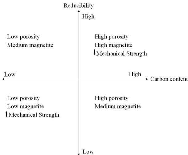
**Figure 5.** Schematic figure of the qualitative trends found in the fired pellets for the tested raw materials.
