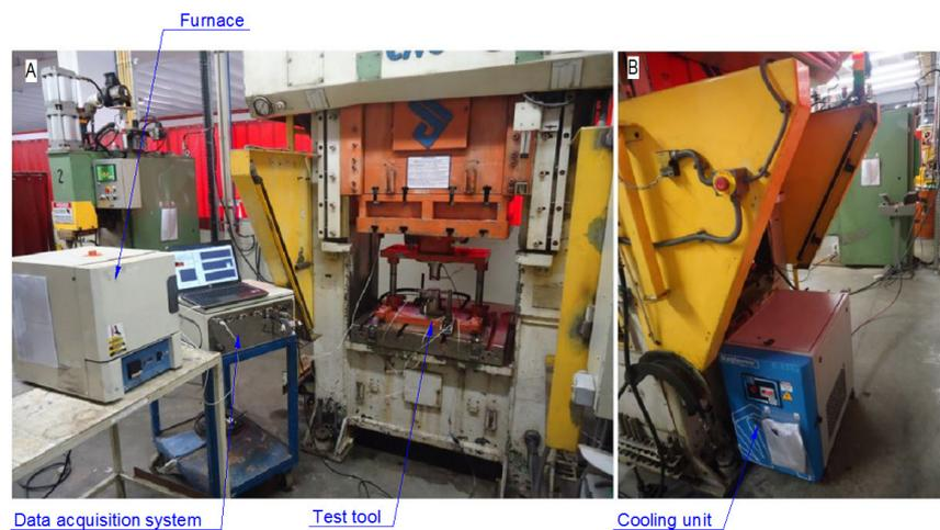
Figure 4. Pictures showing the experimental setup and the equipment used. A) Front view showing hydraulic press with test tool, data acquisition system and furnace. B) Rear view showing the cooling unit.
