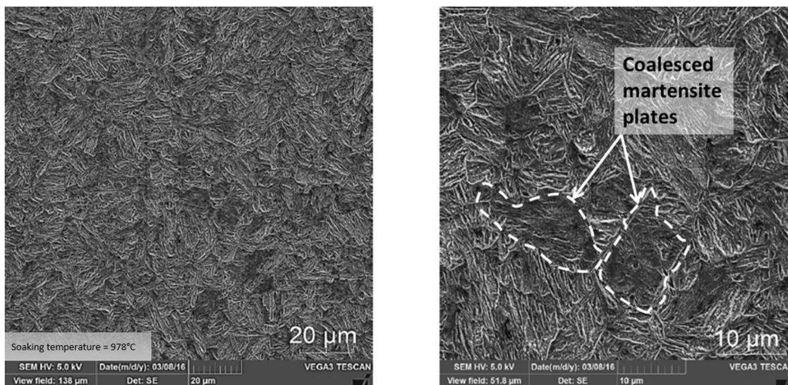
**Figure 9.** Microstructure of the sample processed with polished surface condition.
