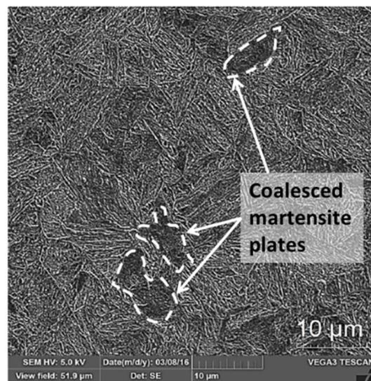
Figure 7. Microstructure of the sample processed with natural surface condition.
