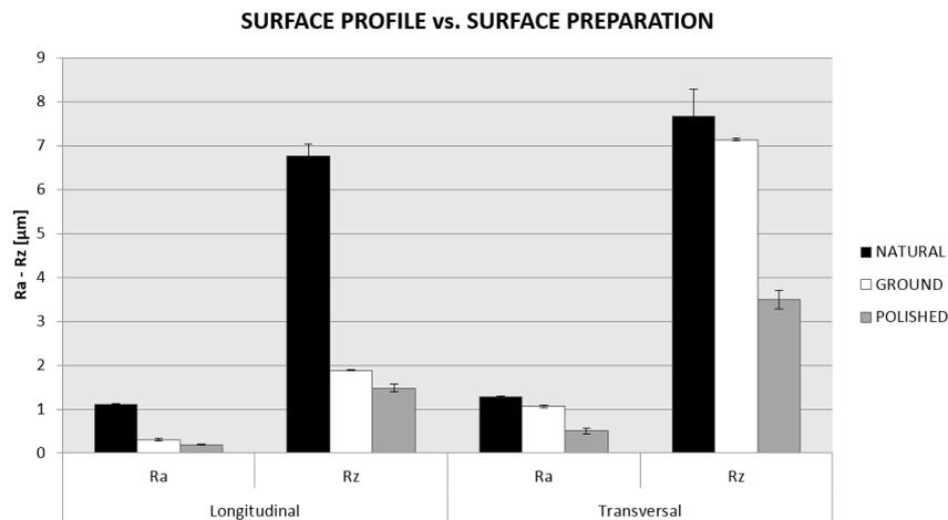
**Figure 5.** Average specimens surface roughness.
