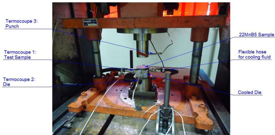
Figure 3. Picture showing the experimental tool and the termocouples.
