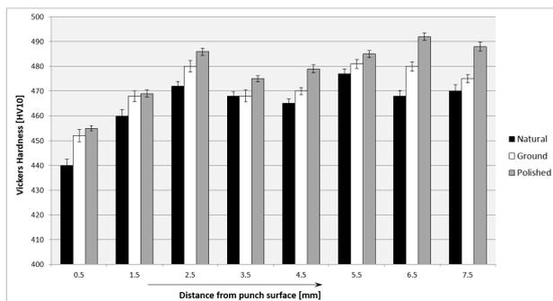
**Figure 10.** HV10 Hardness profile of the samples, starting on the punch side.
