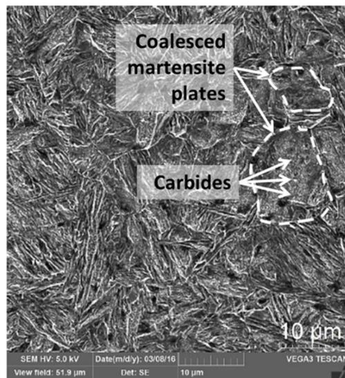
Figure 8. Microstructure of the sample processed with ground surface condition.
