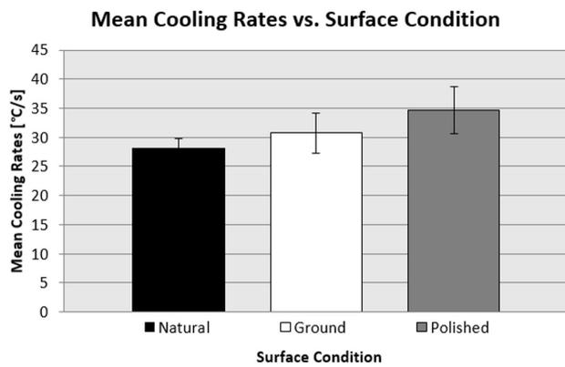
Figure 6. Mean values of the cooling rates for the tested surfaces.
