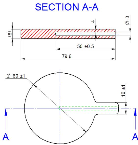
Figure 1. 22MnB5 test specimens geometry.
