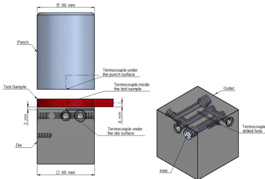
Figure 2. Experimental tool set used in the investigation, showing the position of the thermocouples (on the left) and the cooling channels (on the right).
